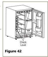
2. If the ice maker is not level, adjust the feet on the corners of the unit as necessary (see **Figure 43**).
